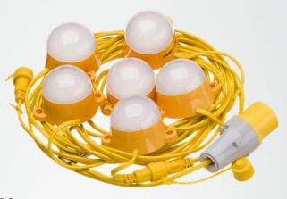
Wattage 30W, 50W, 100W Lumens 3300lm, 5500lm, 11,000lm Lumens per watt 110lm/w CCT 6oook **IP** Rating **IP44 IK Rating** IK<sub>07</sub> Input Voltage: 110V **Power Factor** >0.9 **Dimensions** Length of Festoon: 12m: (30w & 6 way), 22m: (50w & 10 way) 50m: (100w & 20 way) Light: H:60mm Ø75mm **CRI**
