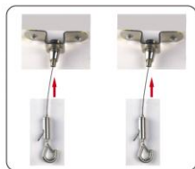
Step 4: Tie the wire rope;
