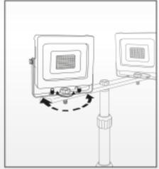
Turn knob anti-clockwise to unlock. Eachflood bracket has a horizontal rotation of 350°, ensure cable doesnot tangle with the stand. Turn knob clockwiseto lock in the desired location.
